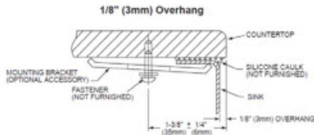
**NOTE: THIS UNDERMOUNT SINK IS DESIGNED TO MOUNT TO SOLID SURFACE (NON-LAMINATE) COUNTERTOP ONLY.**
